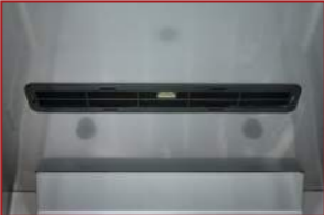
Inlet and exhaust air flow through slits at the top.
