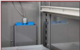
Temp. controlled by sensors located in liquid loaded monitor vessel
